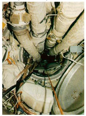
Figure 2. Obstructed hatchway between Mir modules
